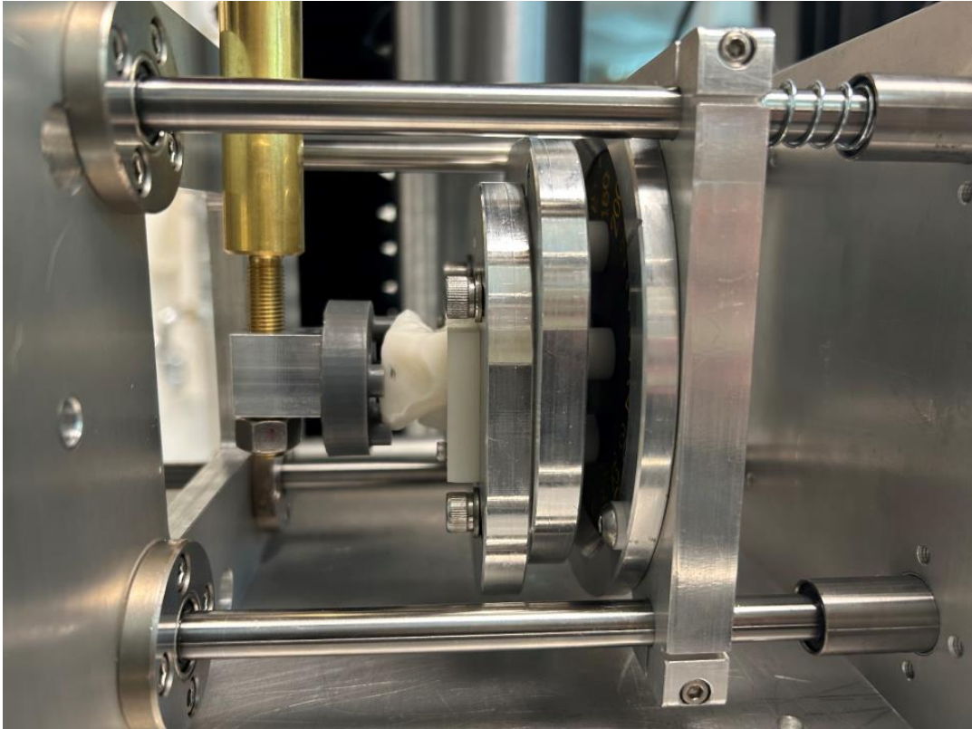
Figure 2: Photo of PSG testing apparatus illustrating the engagement of the PSG with its additively manufactured glenoid model. The PSG is attached to the MTS by a vertical brass shaft while the glenoid model is attached to a low friction horizontal carriage that allows it to be compressed against the PSG using springs to mimic the surgeon's finger force, as well as allowing the glenoid model to shift as the PSG is forcibly dislocated by the MTS.
